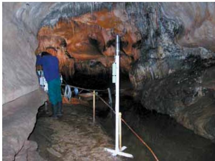
Fig. 11. Radon sensor installed in Domica Cave. Photo. I. Smetanová
