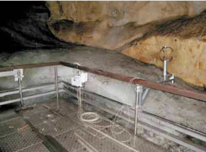
Fig. 2. Different sensors and data logger in ice cave. Photo: J. Zelinka
